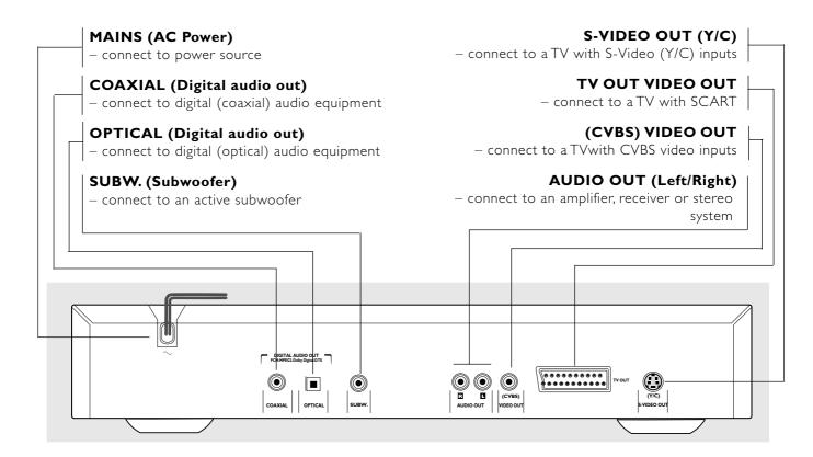
Caution: Do not touch the inner pins of the jacks on the rear panel connectors. Electrostatic discharge may cause permanent damage to the unit.
